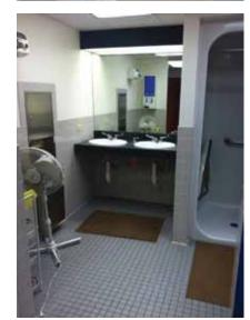
Fig. 2.1.C.4 Mats on the floor provide issues with approaching the accessible lavatory.
