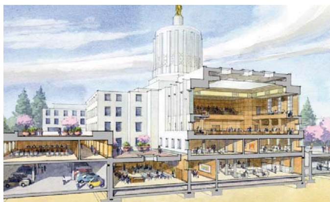
Section through capitol proposed concourse level and additional hearing rooms (Image Credit: Oregon State Capitol Master Plan 2009)
